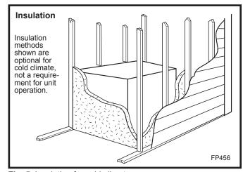
Fig. 5 Insulating for cold climates.
